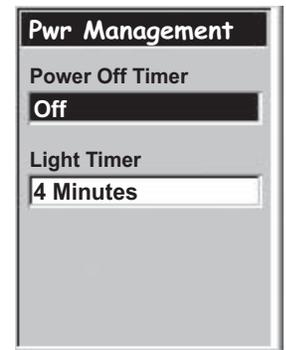
*Note:* When using a GOTO route you should note that if the eXplorist turns off, the GOTO route is erased. If you have a GOTO route activated and you think that the power timer may elapse and turn the eXplorist off, you might want to set the Power-Off Timer to **Off**. This does not apply to multi-leg routes and BackTrack routes.
